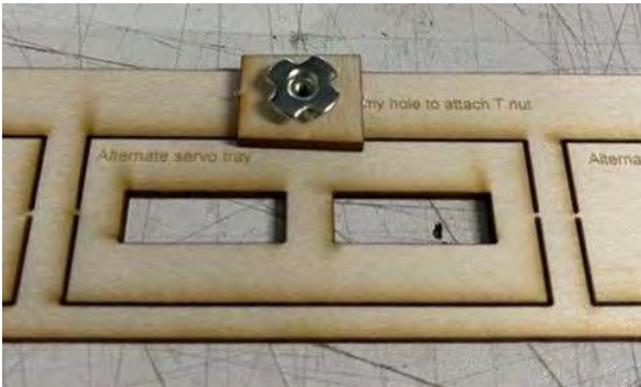
3. Apply thick CA or Epoxy then line up the T nut
