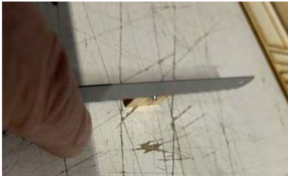
6. Cut off the T nut that passes through the former with a hacksaw blade
