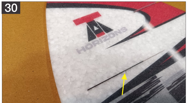
30. Glue the same 3 X 0.5mm Stripe in the slot just behind the rudder horn slot, to reinforce the rudder.
