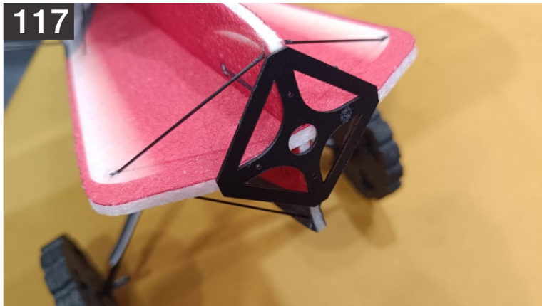
117. Shown above is the motor mount glued, making sure everything is flush and lined up correctly. After that install the motor on it.
