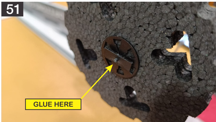
51. Install the wheel over the shaft, make sure it is spinning freely, after this slide in the wheel stopper. Put a small drop of HV CA over the shaft and wheel stopper joint.
