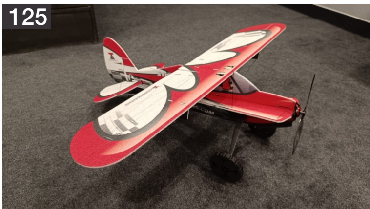
125. Set up your radio as per the suggestions given a little later in this manual, check all the control directions and motor rotation.
