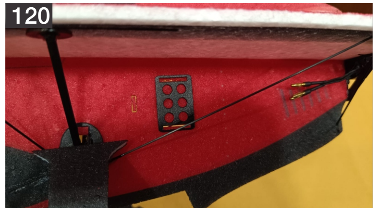
120. Notice above the plate glued onto the side of the fuselage. This can be used to mount the electronic speed controller.
