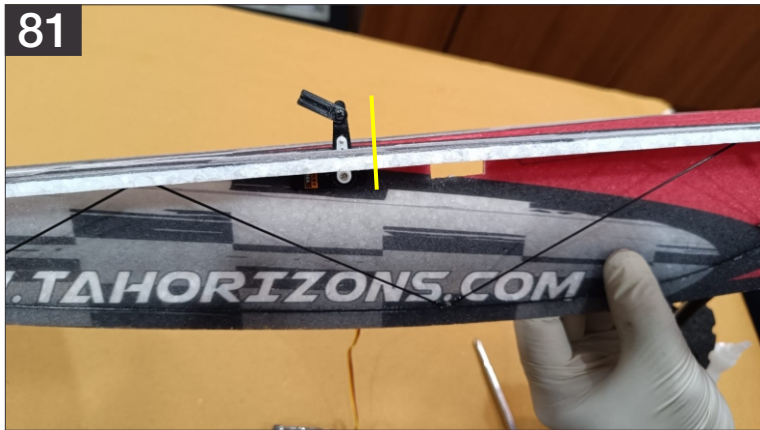
81. Elevator linkage, Make sure you have the servo centered before moving further with the setup, check the orientation shown in the above image.
