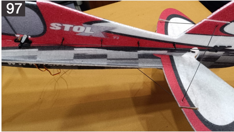
97. Above is the finished linkage setup with rudder centered and rod well fitted and glued in both the quick links with all the guides in place. Use the same process like we did in previous linkage setups.
