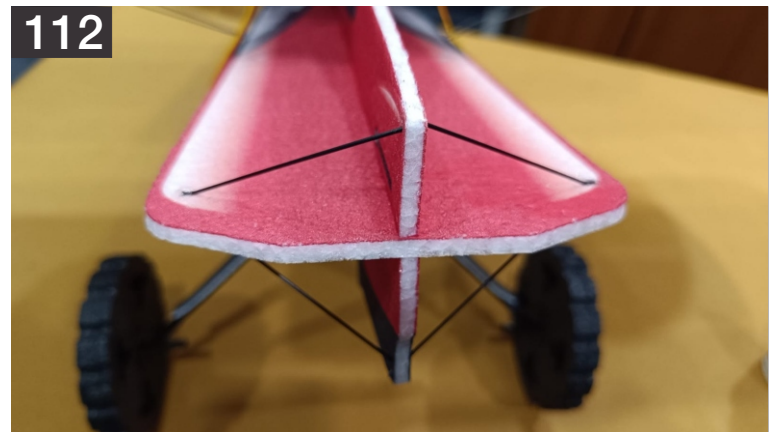
112. Here are all the mount reinforcement rods glued in place.
