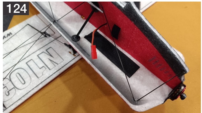
124. The long piece of velcro along with the strapping velcro mounted, above is the location of the battery for this setup.
