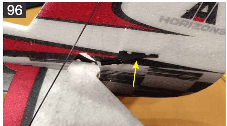
96. Install the rudder horn in place. (Opposite side of the elevator servo).
