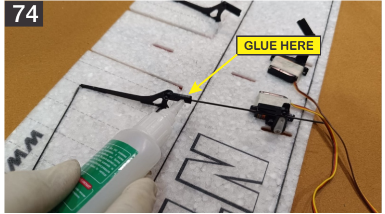
74. Locate the 100mm aileron control rod, glue it on the one side, using thin CA or optionally HV CA. Make sure you have servo arm centered.
